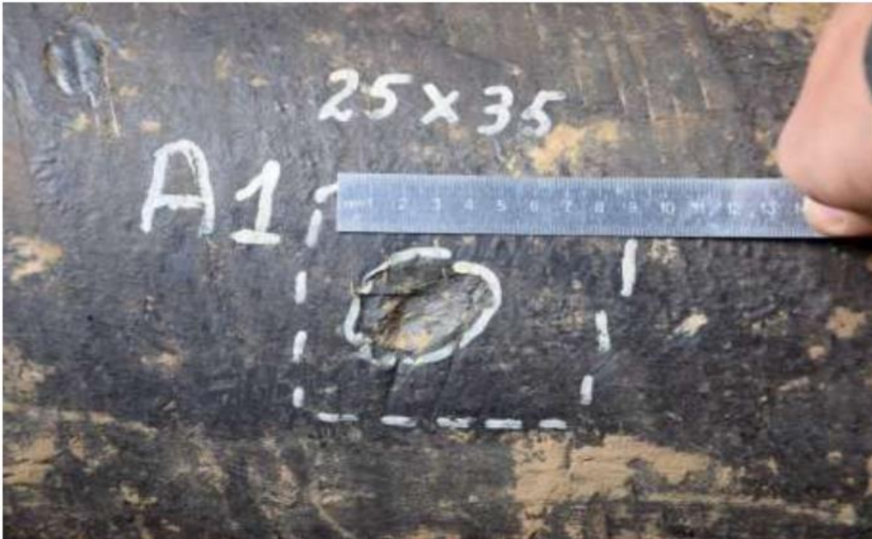
Figure 1. Damaged coating (A1 dent 25x35x6 mm)
