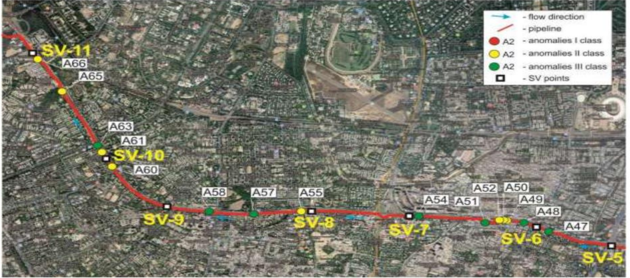
Figure A3.42. Scheme of localized anomalies (Stress Concentration Zones) at the « DESU-Maruti » pipeline
