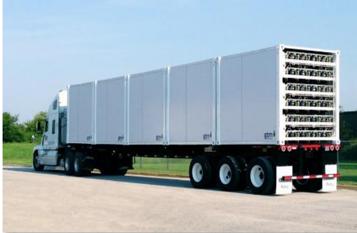
Gas Transportation Modules
