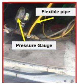
Makeshift Arrangement of Flexible Fitting alongside Pressure Gauge CNG Cylinder.
